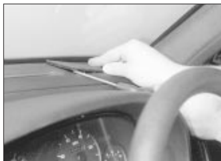
21.9a Prise the loudspeaker from the fascia . . .
