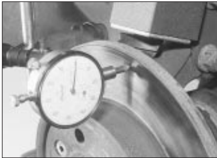
7.4 Checking disc run-out using a dial gauge
