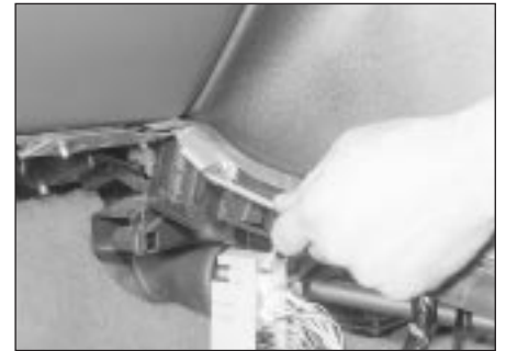
30.69 . . . and the rear centre facia securing bolts
