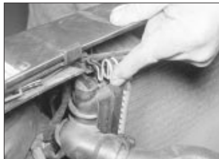
3.10 Releasing a radiator upper securing clip
