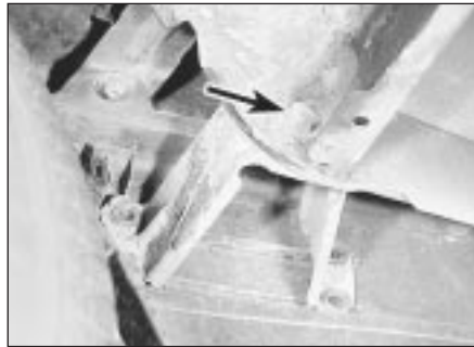
6.4 Front bumper side securing bolt (arrowed)
