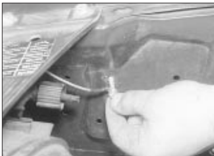
11.8 Unbolt the earth leads from the corners of the engine compartment
