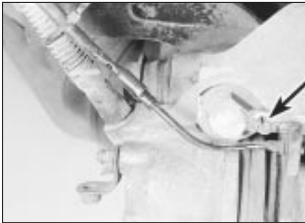
4.5a Extract the spring clip (arrowed) . . .
