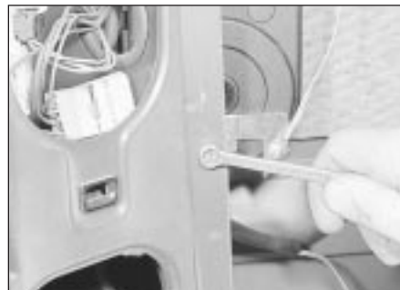
22.18b Unscrew the aerial motor securing bolt . . .
