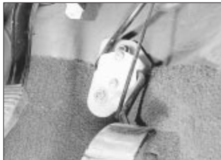
8.2 Accelerator pedal pivot bush
