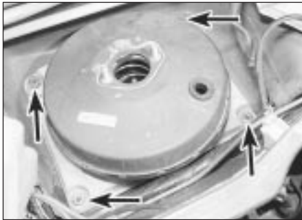
15.14 Unscrew the nuts (arrowed) securing the servo to the scuttle
