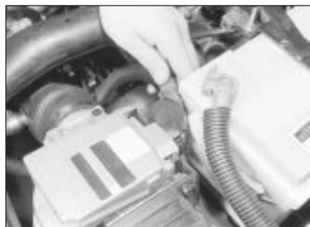
2.1 Disconnecting the airflow meter multi-plug (Bosch L3.1-Jetronic)
