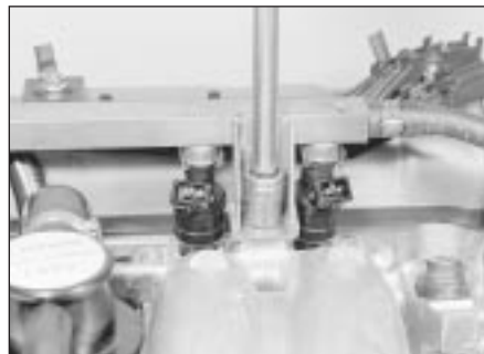
14.28a Removing a fuel rail bolt . . .
