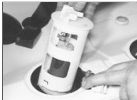
9.12a . . . then lift out the fuel pump . . .
