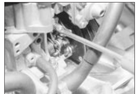
10.4b Idle speed adjustment screw
