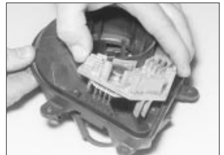
9.68b . . . and withdraw the control module
