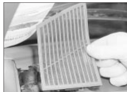
21.6 Remove the loudspeaker cover panel from the top of the fascia . . .
