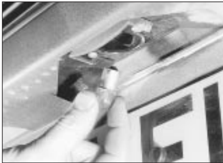
5.40 . . . and withdraw the number plate light bulb - Saloon model
