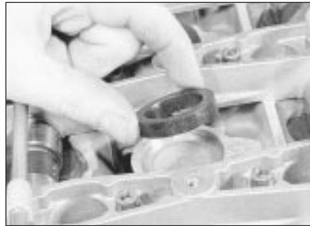
4.32 Fitting a spark plug hole oil seal
