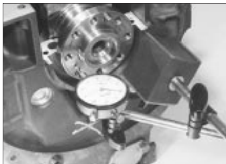
14.2 Checking crankshaft endfloat using a dial gauge
