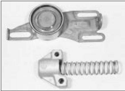
8.31 Timing belt tensioner assembly components - early 1580 cc and 1905 cc 8-valve models
