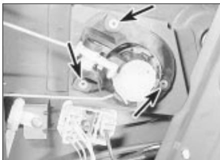
19.4 Tailgate lock cylinder securing rivets (arrowed)
