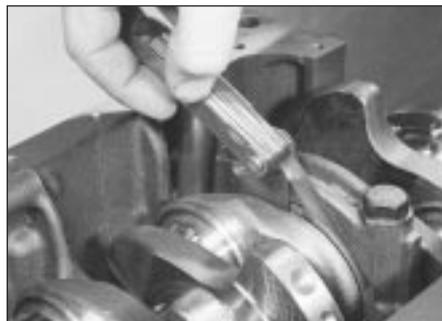
14.3 Checking crankshaft endfloat using feeler gauges
