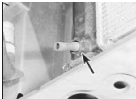
20.3 Radiator drain outlet (arrowed)
