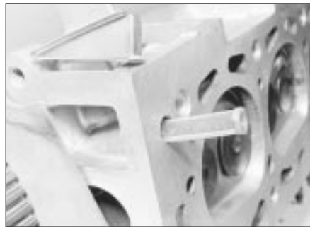
7.8 Oil filter partly withdrawn from the oil gallery in the cylinder head
