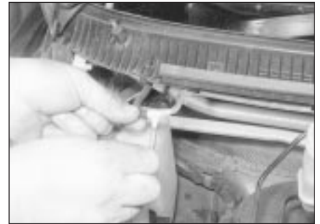
25.8 Disconnect the washer fluid hose
