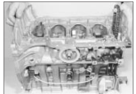
18.44 . . . then lower the main bearing ladder into position
