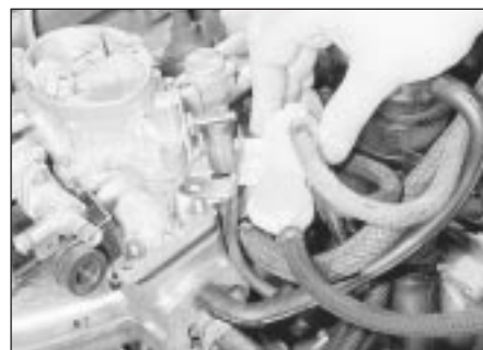
12.9 Lifting off the fuel reservoir
