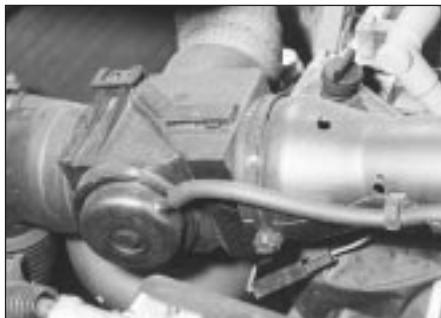
3.17 Air temperature control valve assembly (TU engine)
