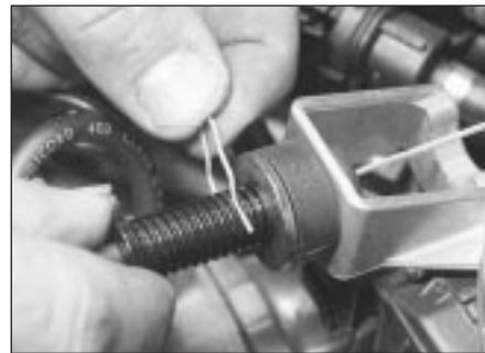
4.3 Adjust the accelerator cable as described in text
