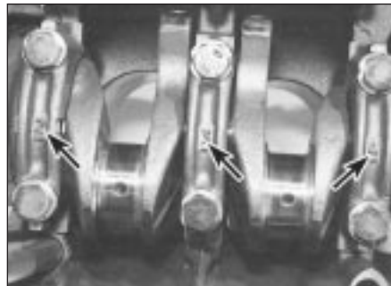
11.17 Main bearing cap identification markings (arrowed)
