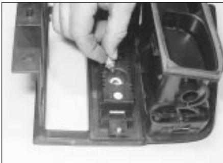
6.23 Removing the clock illumination bulb - models from 1993
