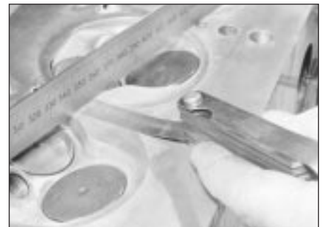
8.6 Checking the cylinder head gasket surface for distortion
