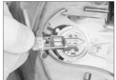
5.23b Removing a headlight-mounted driving light bulb
