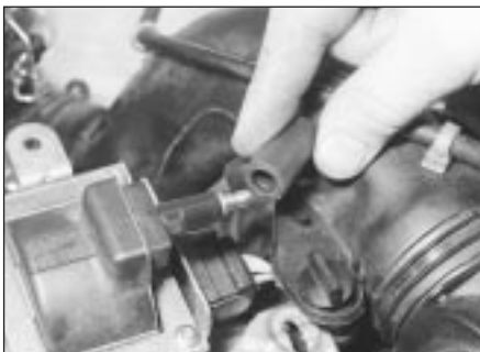
3.4a . . . then disconnect the HT lead . . .
