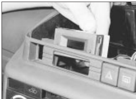
11.5 Removing the clock - models up to 1992
