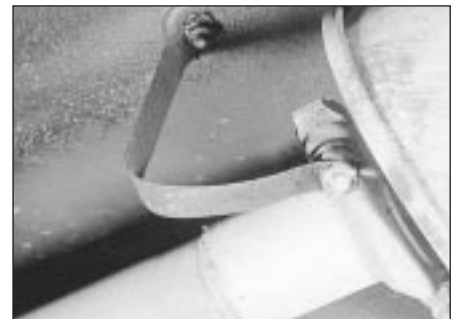
16.1 Exhaust-to-floor panel earth strap fitted to early models
