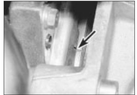
6.2b Timing marks on the flywheel and timing plate
