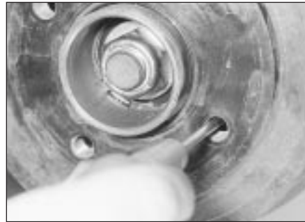
9.3b Releasing the handbrake operating lever
