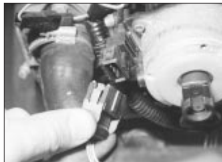
4.3a Disconnect the distributor wiring connector . . .
