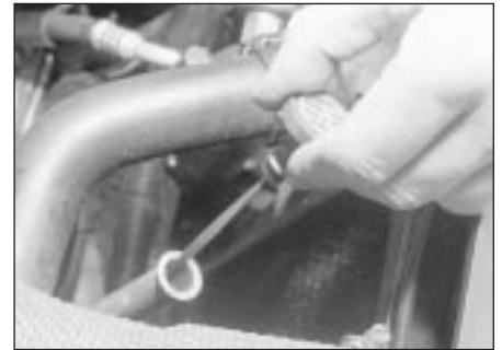
4.2a Withdrawing the automatic transmission dipstick
