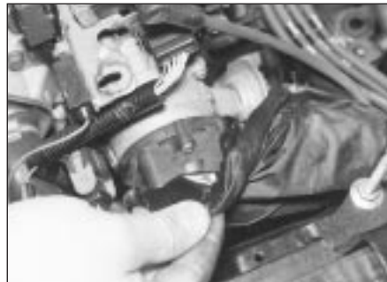
4.2a Peel back the waterproof cover . . .
