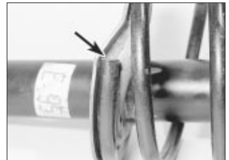
5.10b . . . making sure the lower end of the spring locates against the stop (arrowed)
