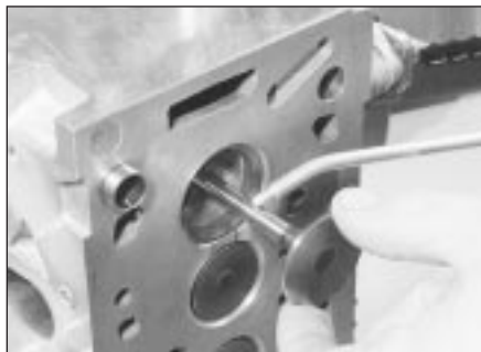
9.1 Lubricate the valve stems prior to refitting
