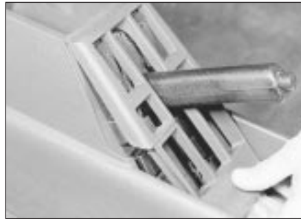
4.20 . . . then prise off the switch trim panel . . .
