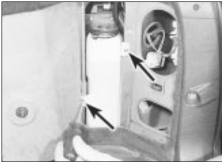
19.8a Remove the two securing screws (arrowed) . . .
