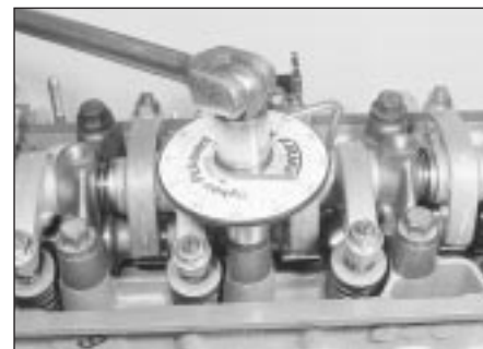
11.38 . . . then through the angle specified for stage 2
