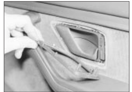
13.2 Removing the door interior handle surround
