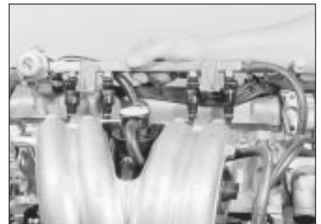
14.28b . . . and pulling up the rail and injectors
