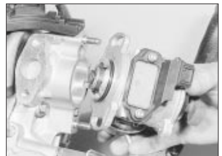
4.4c . . . and withdraw the distributor from the cylinder head
