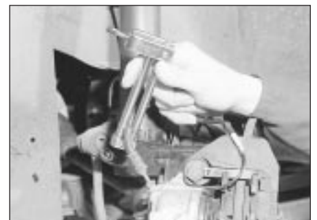
10.2 Using a clamp on the caliper hydraulic hose
