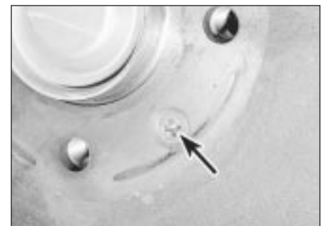
9.2 Rear brake drum retaining screw (arrowed)
