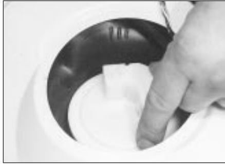
10.1 Removing the fuel gauge sender unit
