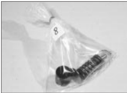
7.7 Place each valve and its associated components in a labelled polythene bag
