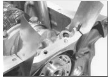
18.73a Fitting No 1 main bearing cap, using metal strips to retain the side seals
