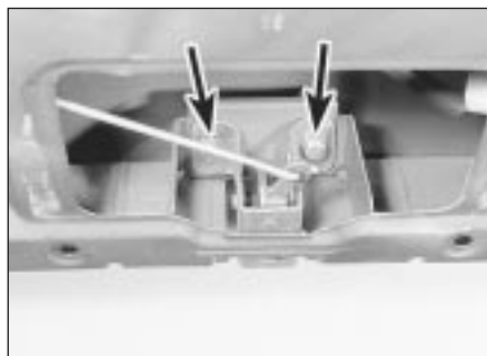
19.9 Tailgate lock securing bolts (arrowed)
