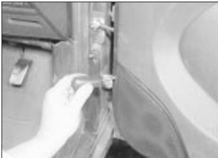
13.3 Removing a loudspeaker cover panel securing screw
