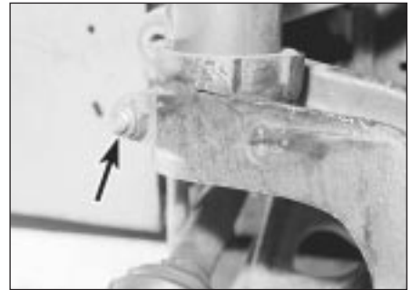
2.12 Hub carrier-to-suspension strut clamp nut (arrowed)
