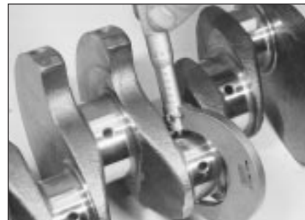
14.10 Measuring a crankshaft big-end journal diameter
