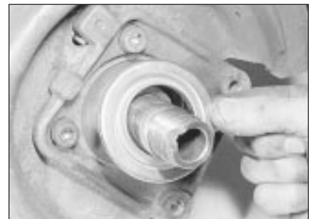
10.6c . . . and the oil seal support cup
