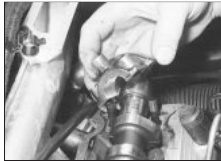
10.32 . . . and remove the camshaft bearing caps . . .
