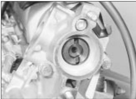
4.10 Off-set drive slots on the camshaft
