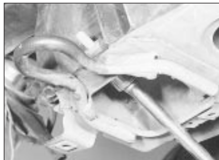
11.12 Removing a body front panel lower securing bolt
