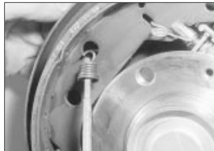
6.6b Removing an early type Bendix shoe retainer spring
