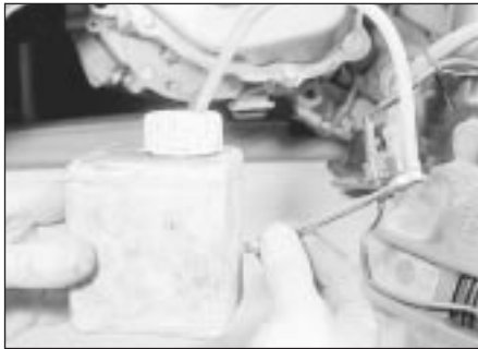
2.20 Using a one-man brake bleeding kit on a front caliper
