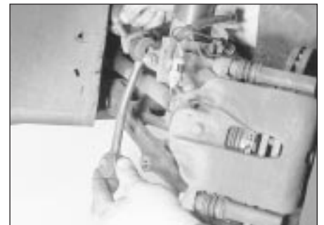
8.3 Removing an anti-roll bar drop link
