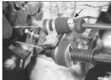
9.10 Choke cable-to-rubber collar retaining clip (arrowed)
