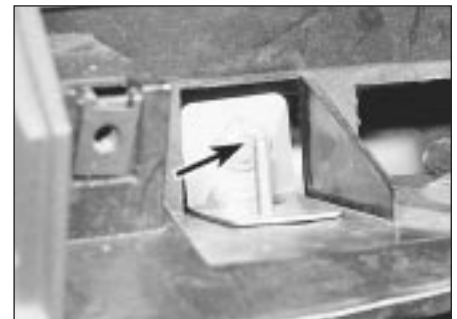
30.23 Upper facia securing bolt (arrowed)
