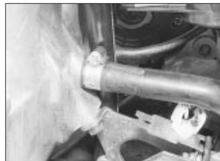
18.6 Supplementary air device air hose connection on inlet manifold
