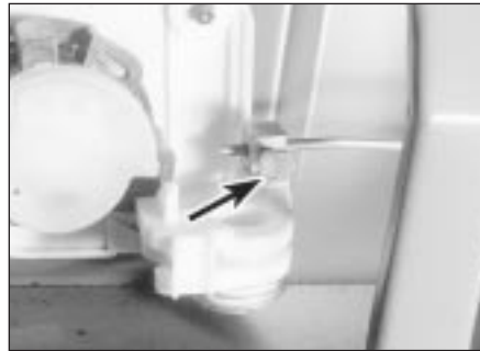
17.4 Unscrew the lock operating rod pinch-bolt (arrowed)
