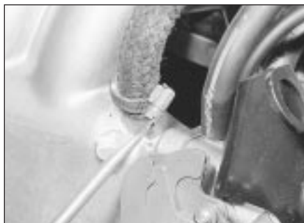
18.3 Disconnecting the brake servo vacuum hose
