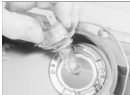
5.4b . . . then withdraw the headlight bulb
