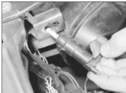
7.4 Removing a cable-operated headlight adjuster
