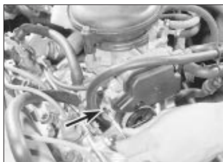
10.7 Idle mixture adjustment screw (arrowed)
