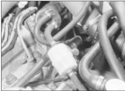
8.1 Fuel filter location on carburettor models
