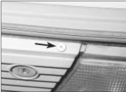
17.3 Drill out the rivets (arrowed) from the body rear trim panel
