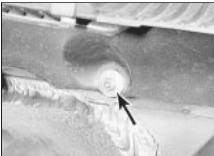
30.20 Facia securing nut (arrowed) in scuttle
